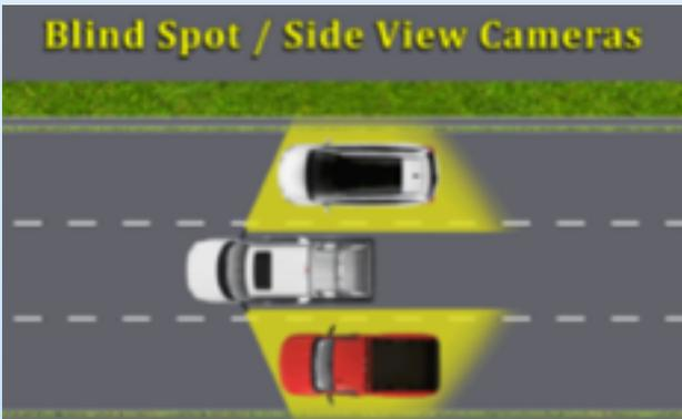
The Blind Spot or Lane Departure Cameras (Right & Left) will be displayed on the radio screen automatically whenever the turn signal indicator is activated. A configurable 12 second timeout or continuous operation
