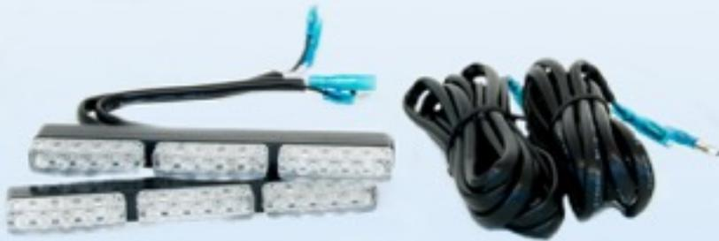
These universal Driving Lights feature a 3M backing that will fit any vehicle or body kit. These aftermarket Driving Lights harness the power of LEDs to provide a crisp, bright light while using minimum power and producing almost no heat. The ArmorBeam Model A Driving Lights feature 15 LEDs in each housing.
